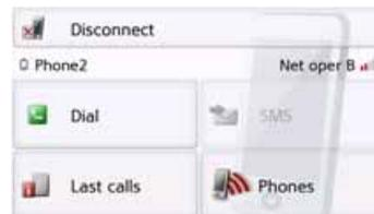
In the upper area of the telephone menu, the signal strength of the cell phone, the charging level of the cell phone, the telephone name and the network provider are displayed, if available.
