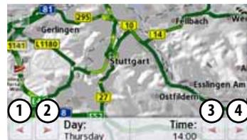
You can determine the expected flow of traffic by the colour of the road. Green signifies a clear road, red signifies congestion. All possible colours are displayed on the right-hand side of the screen.
