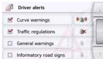
The available driver alerts are divided into 4 categories. The four categories can be enabled  or disabled  individually. The warning sound can be set individually for each of the four categories by pressing the symbol with the bell (
