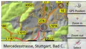
> Then press any point on the map and move it in the required direction. The map is then moved accordingly.
