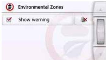
You can let yourself be warned about environmental zones provided that this information is saved in the card material and is supported by your navigation system. This function can be activated  or deactivated . By pressing the symbol with the bell, you can set the audible warning signal (
