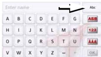
> Press repeatedly on the button in the top right-hand corner of the display until the desired method of entry is activated.
