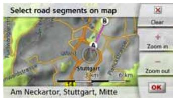
> Define the start and end point of the section to be blocked by touching the map.
