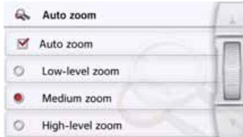
Pressing the **Auto zoom** button switches the zoom function on () or off (). When the zoom function is switched on, you can select whether the autozoom action should be weak, medium or strong.
