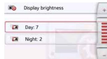
> Use the **-** and **+** buttons to set the desired brightness for the day and night display.
