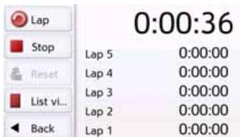
> Press the **Lap** button to stop the current recording and start a new lap recording.
