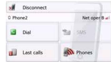
If Bluetooth is not activated upon calling up the telephone function, the system will prompt you to switch Bluetooth on.
