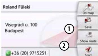
Press the **Start** button to begin route guidance to the address displayed for this contact straight away.
